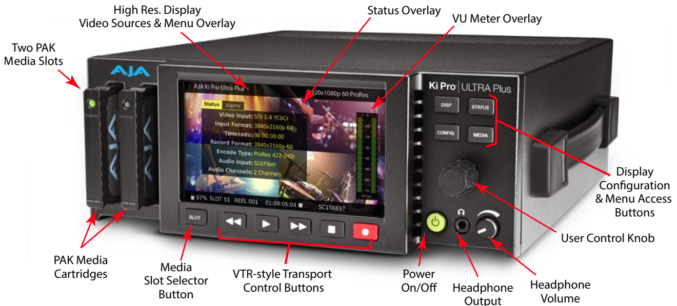
Figure 1. Ki Pro Ultra Plus Operator Side Controls
